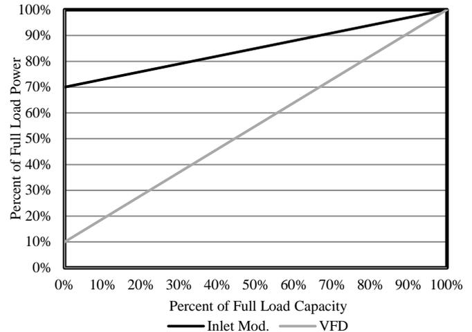
*Figure 1. Illustration of power percentage vs. capacity percentage for inlet modulation and VFD control schemes.*
