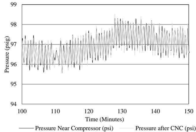
Figure 3. Illustration of pressure drop with 50 minutes of data logging for two points in the facility; near-compressor and after CNC.
