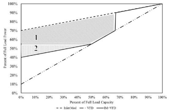
Figure 6. Areas of Savings from Inlet Modulation and VFD System
