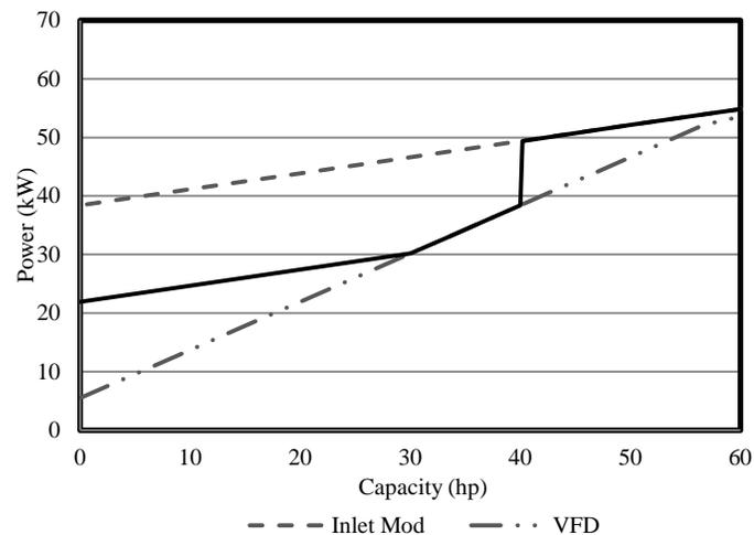
Figure 4. Illustration of Full Load Power vs. Percent of Full Load Capacity.
