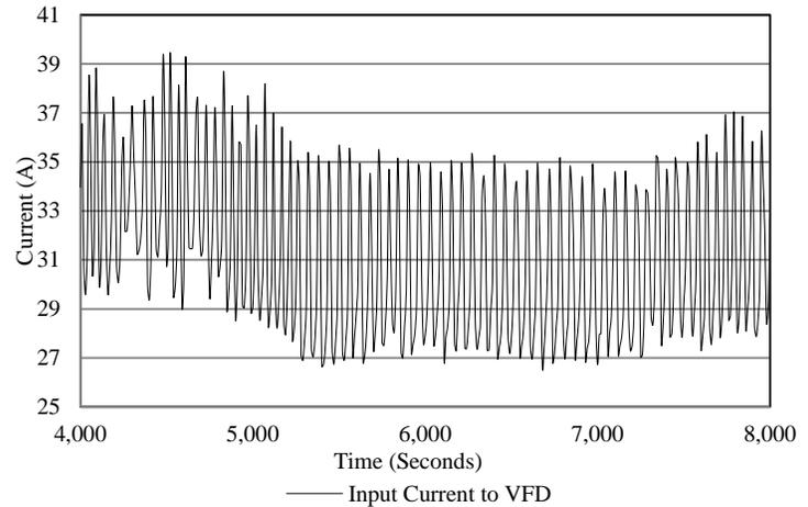
Figure 5. Illustration of current draw of one of the 60 hp compressors.
