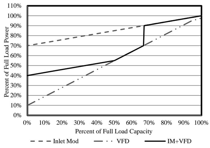
Figure 2. Illustration of Full Load Power vs. Percent of Full Load Capacity.
